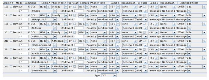
The matching SignalMan configuration is shown here. You may note that there is no 'Dark' entry. If it is required, then you could add this 9th item on the next 'Masts' pane, or simply replace an unneeded aspect in this list.
