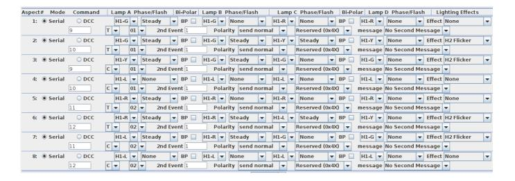
Aspect #3 (9C Clear) is simpler in that it just flashes the red LED 'H1-G Steady' in 'Lamp B' followed by the green LED 'H1-Y Steady' in 'Lamp A'. The 2 unused lamp entries are set to 'None'.
